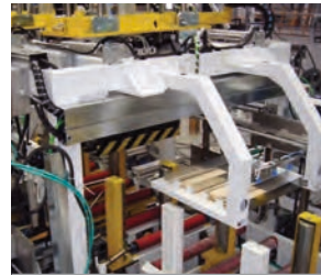
Fully automatic strapping machine with steel strap and automatic insertion of wood on the 4 sides of the bundle.
